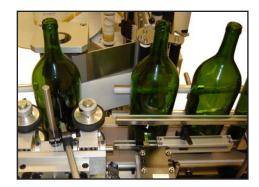
This technically-advanced labeling system was designed specifically for wineries with challenging export business. It has the ability to 'over-label' or apply new labels directly over existing labels. This system is also capable of handling unlabeled bottles.
