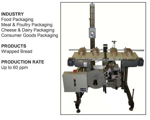
These integrated labelers feature Quadrel's high speed Q65 wipe-on label applicators. Products are conveyed on a dual split belt, food-grade conveyor with a powder coated carbon steel frame.
