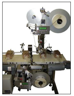
The system shown on the left is used for bottom apply only but an additional head support was added to provide flexibility for future use of a top apply labeler.
